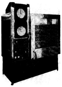
This atmosphere control cabinet is designed by Package Materials Laboratories for testing products in various environments of temperature and humidity. The device has a range of 18% to almost 100% relative humidity and temperature variation from 20° to 200° F. PE 7
